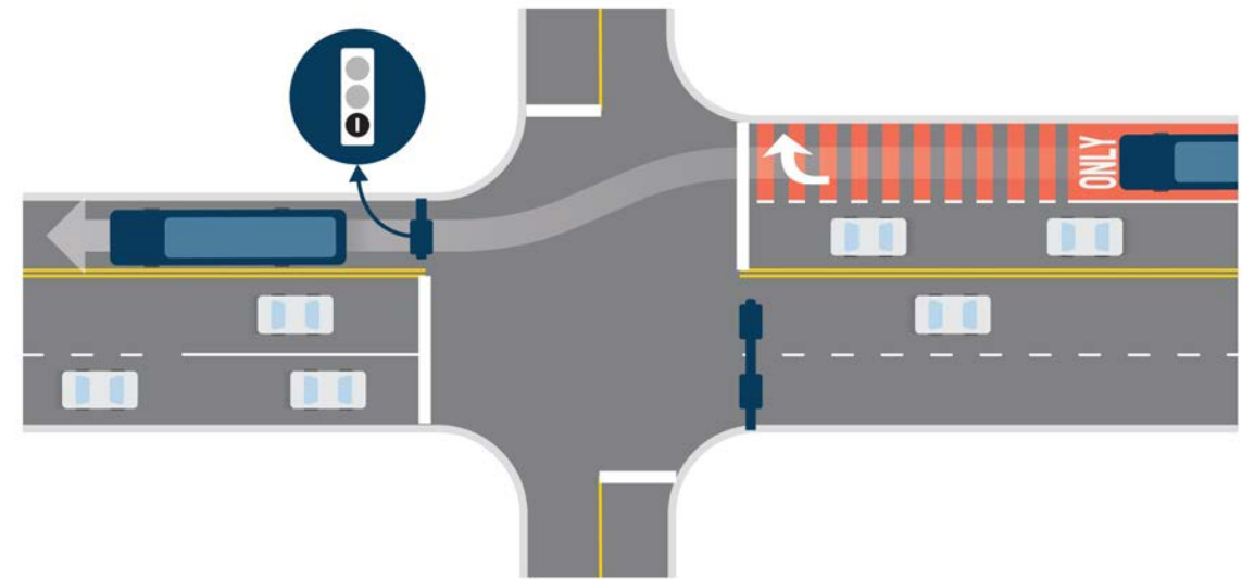
A queue jump signal is needed when there is no approach lane across the intersection.
